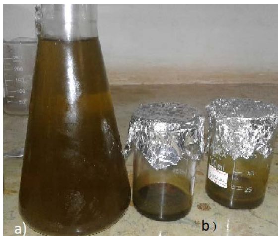
Fig. 2 Extraction of oil from filter cake by using dissolvent extraction method a) Leaching extraction Cold Solvent & Sugar cane filter cake oil b) Sugar cane filter cake oil extracted
